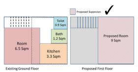
In case, there is not enough space on the ground floor, enhancement can also be carried out on the first floor; provided that the Structural Safety
