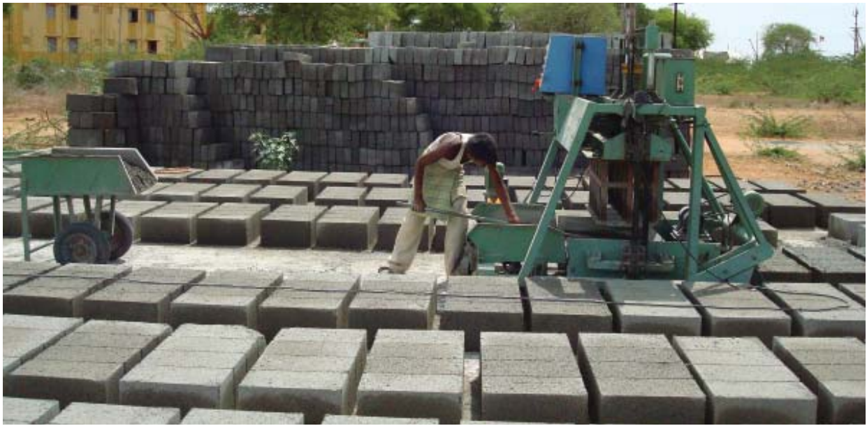
On-site production of Flyash Blocks during the construction of Demonstration Houses under VAMBAY at Trichi, Tamil Nadu
