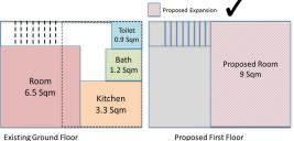
In case, there is not enough space on the ground floor, enhancement can also be carried out on the first floor; provided that the Structural Safety is ensured.
