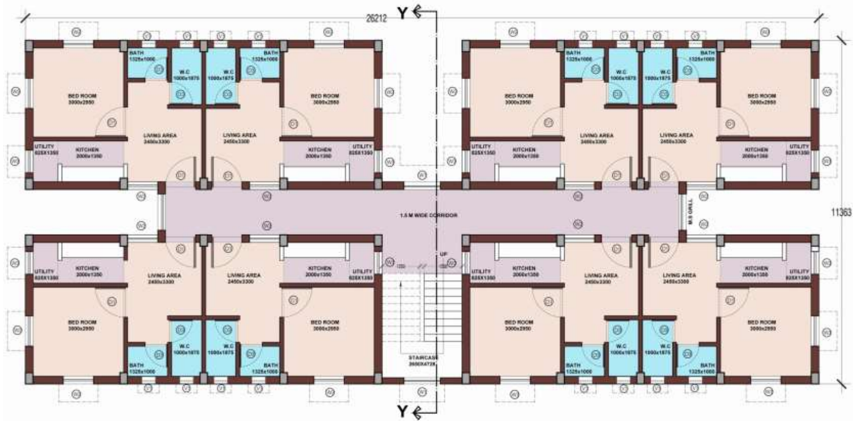
TYPICAL GROUND 1ST,2ND & 3RD FLOOR PLAN BLOCK-A BUILT-UP-AREA =272.4 SQ.M (all dimension are in mm)
