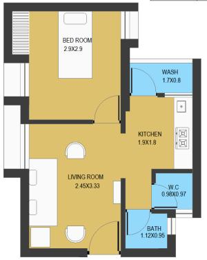
BUILT UP AREA OF TYPICAL UNIT =30.75 Sq.Mt. CARPET AREA OF TYPICAL UNIT =25.02 Sq.Mt.
