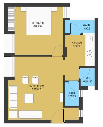
BUILT UP AREA OF TYPICAL UNIT =41.65 Sq.Mt. CARPET AREA OF TYPICAL UNIT =35.15 Sq.Mt.
