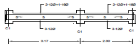
DETAIL FOR BEAM PB/RB-7 to PB/RB-12
