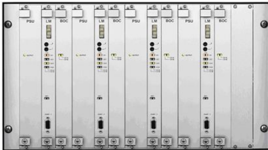
Figure 8 Lineside Electronic Unit (LEU)
