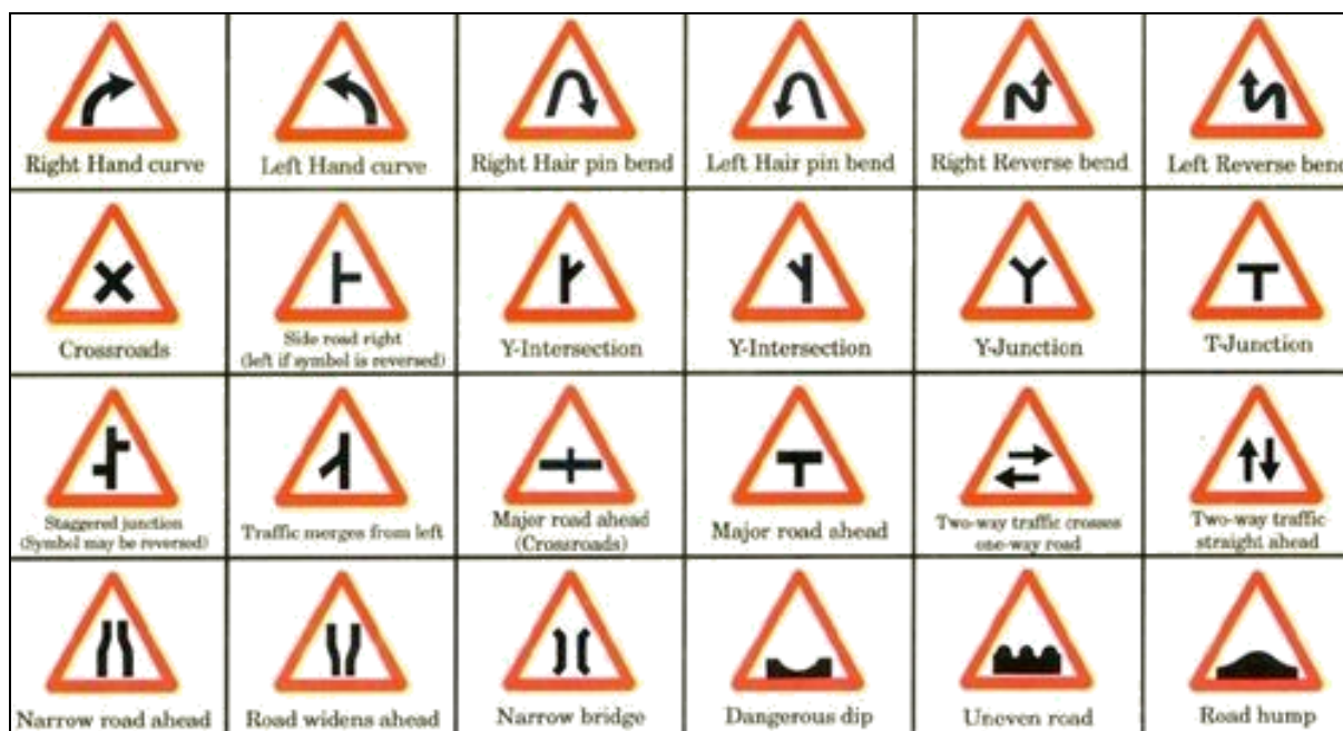
FIGURE 5-29: CAUTIONARY OF WARNING SIGNS
