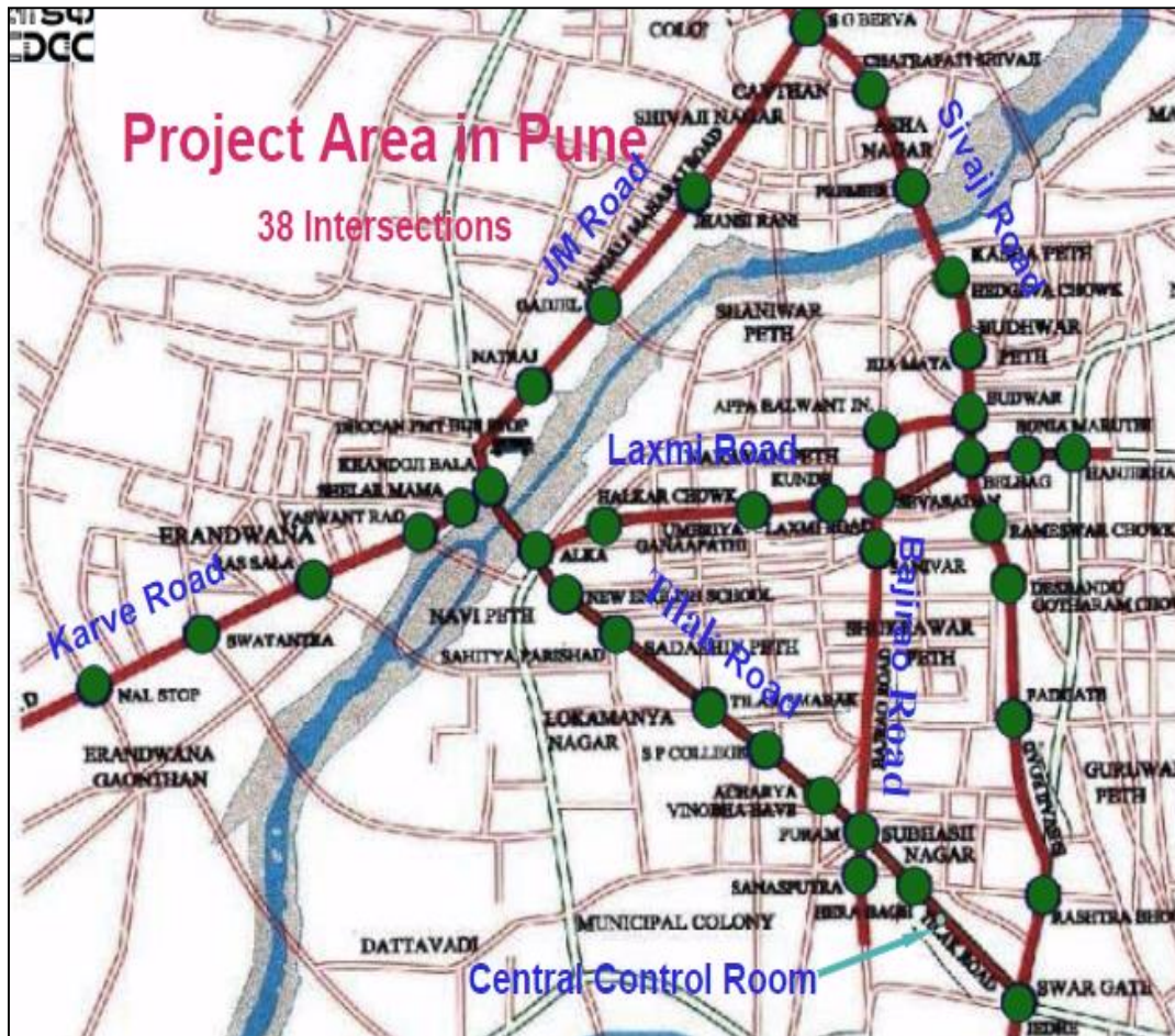
Figure 60 ATCS PROJECT JUNCTIONS IN PUNE
