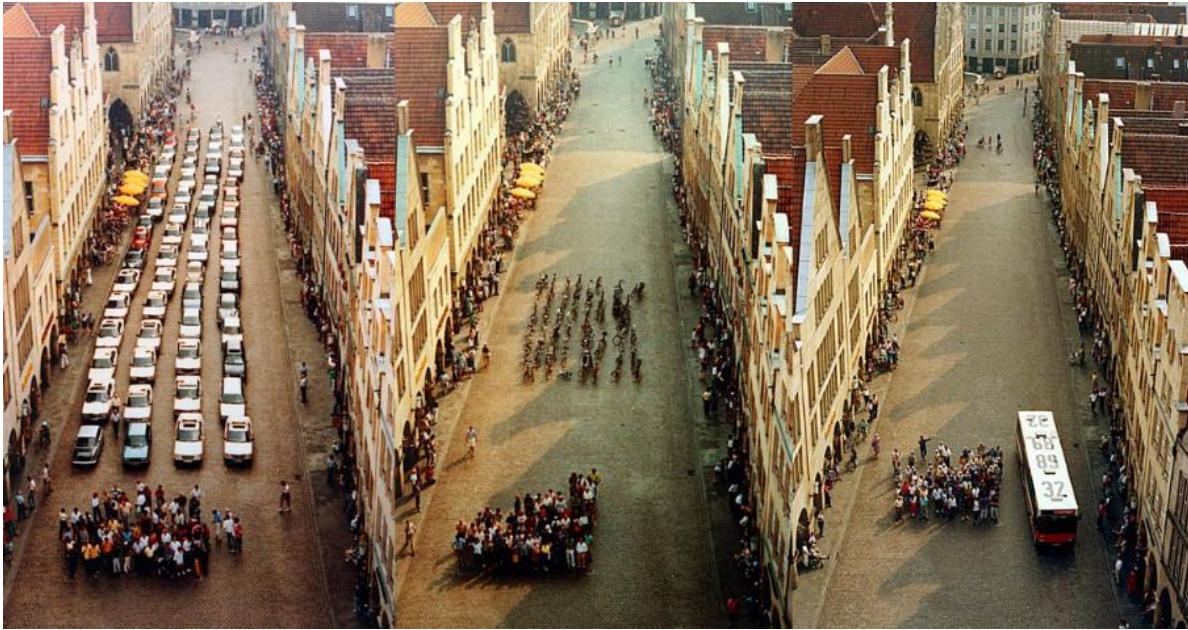
Figure 33 THE AMOUNT OF SPACE REQUIRED TO TRANSPORT THE SAME NUMBER OF PASSENGERS: CAR, BICYCLE, AND BUS. 10
