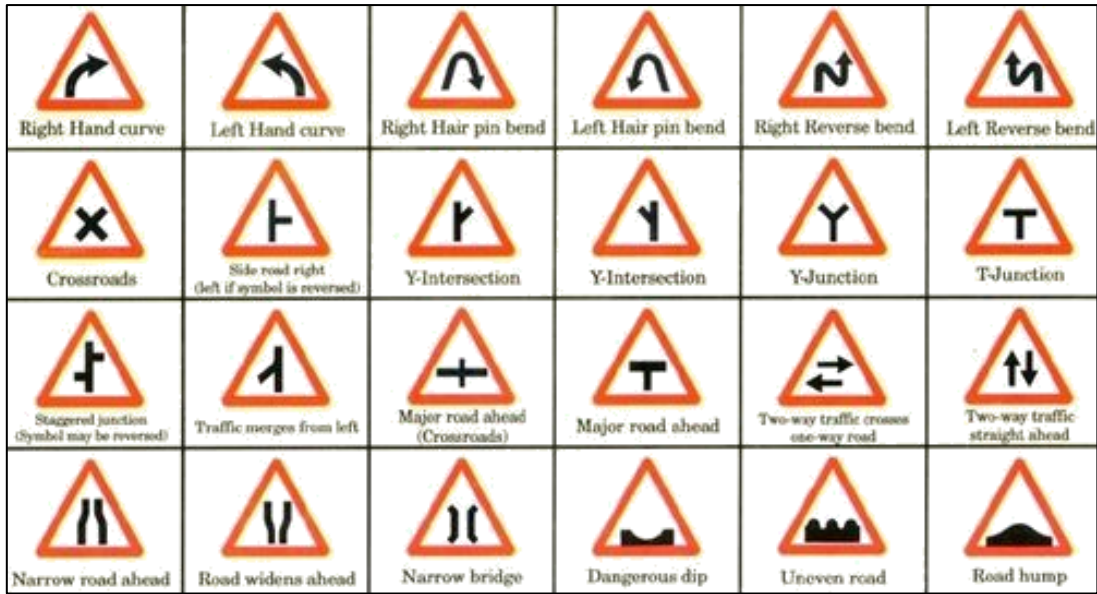
Figure 5.5-9 CAUTIONARY OF WARNING SIGNS
