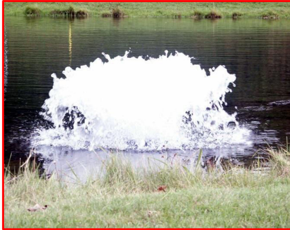
Figure 10.2: Surface agitation can be achieved by Aerators or by Pumps/blowers
