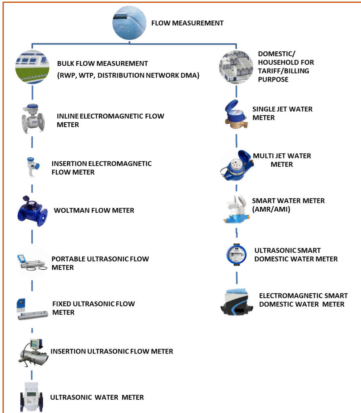
Figure 13.1: Classification of Water Flow Meter based on consumer category
