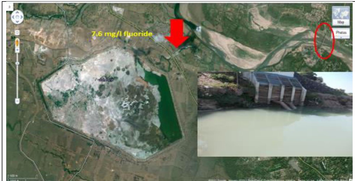
Figure 1: Ash Pond in the Catchment of Kanhan River (Intake well of Kanhan WTP encircled, and change in colour of water due to overflow of breached ash pond in February 2017)
