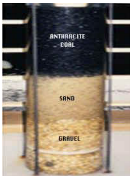
Figure 8.68: Pilot plant for Dual Media Filters
