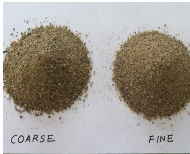
Figure 8.72: "Coarse" and uniform OCW, media is used in MMDB filters
