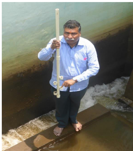
Figure 8.69: Checking media expansion during backwash using sand expansion stick
