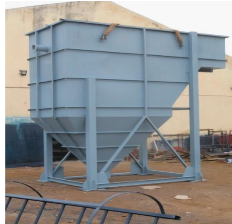
Figure 8.39: Small Capacity Plate Settlers unit (at Bhopal in India)
