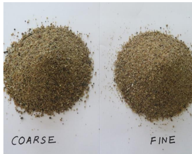
Figure 8.42: 'Coarse' and Uniform OCW, Media is used in MMDB filters
