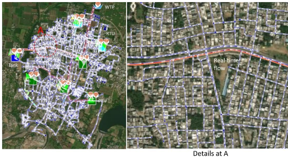
Figure 14.21: Real-time Simulation of flow in network
