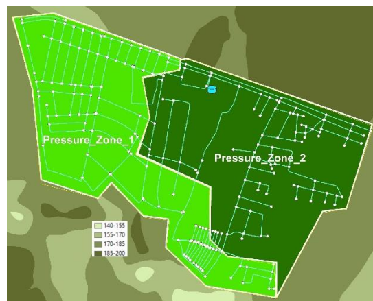
Figure 7: Marking existing pipe network in pressure zones
