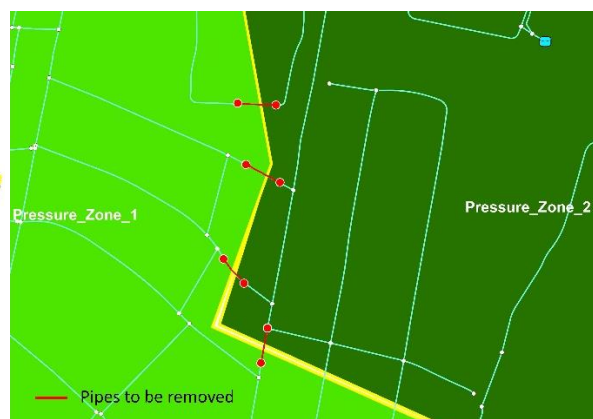
Figure 9: Retrofitting required to remove the cross connections
