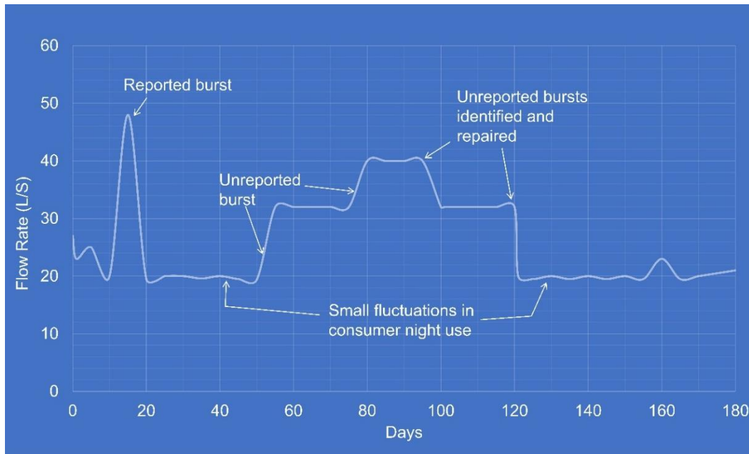
Figure 12.31: Fluctuation in MNF over 180 days
