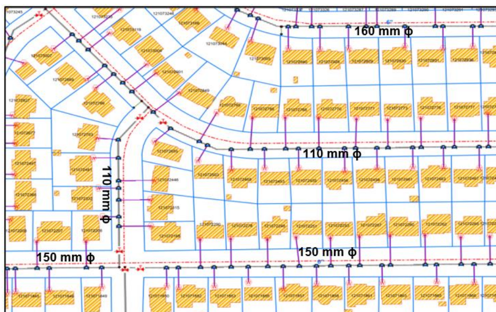
Figure 5: GIS: Integration of Water Network with Consumer database
