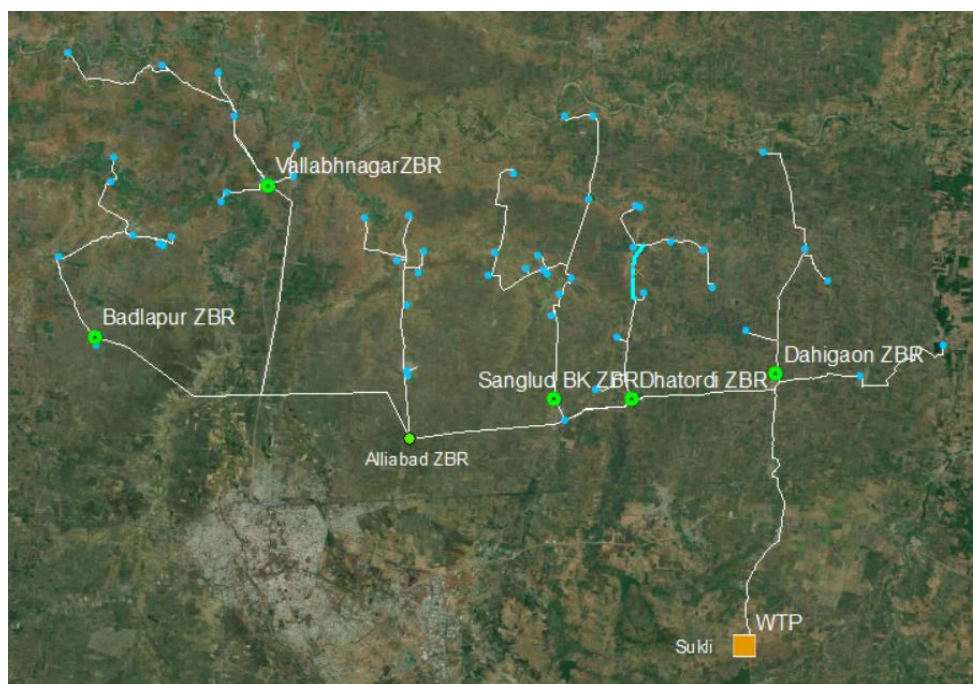
Figure 1: Configuration as per accepted tender of sanctioned scheme. (ZBRs are shown in green colour and village ESRs in blue colour)
