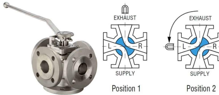
Figure 11.103: Four-way design of Multi-Port Plug Valves
