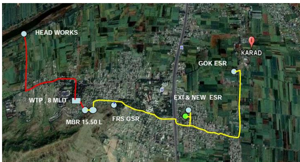
Figure 1: Malkapur 24×7 water supply system
