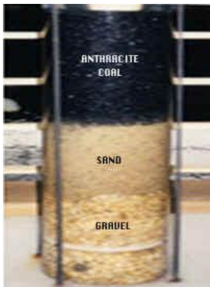
Figure 8.38: Pilot Plant for Dual Media Filters
