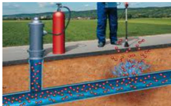
Figure 4.6: Detection of Leak through Gas
