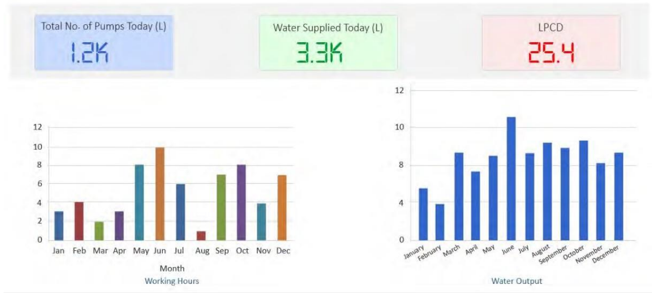
Figure 7.4: Typical Dashboard for Water Pump – Remote Monitoring System
