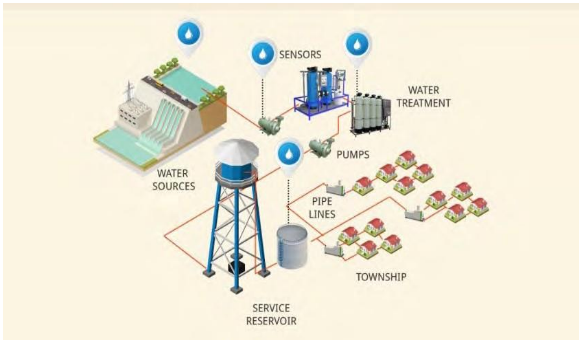
Figure 7.6: Measurement & Monitoring of Water Service Delivery
