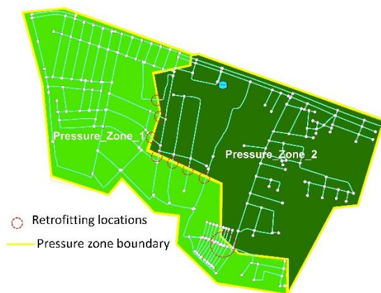
Figure 8: Retrofitting required to separate out pipe from pr. zones
