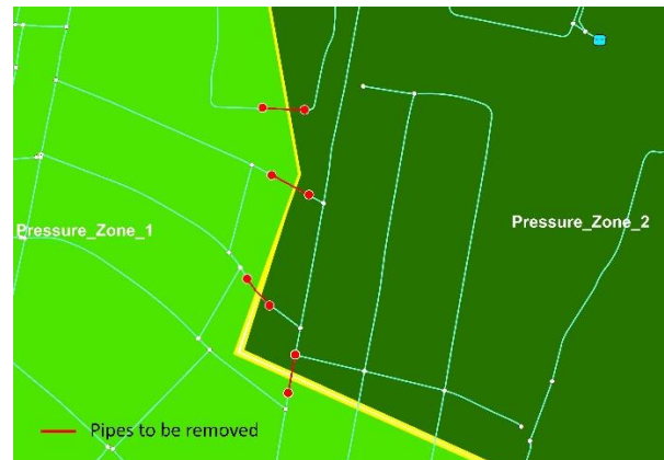
Figure 9: Retrofitting required to remove the cross connections
