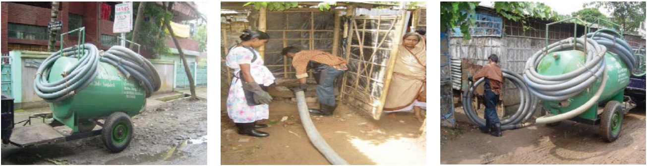
FIGURE 3.2: The Vacutug being used to desludge a cesspool
