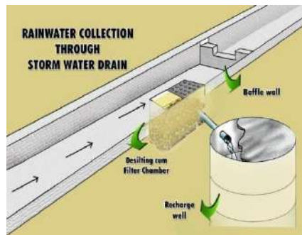
Figure 9.5: Rain Water Collection through storm water drains
