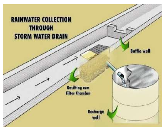
Figure 9.6: Rain water collection through storm water drains
